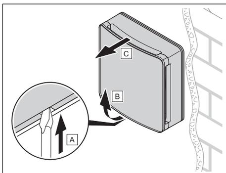
3. Remove the fan unit with wind guard and front panel.
